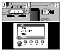
(1) Set the Mode switch to " $\mathbf{E}$ ". 2 Press the "MENU/OK" button to display the Menu screen on the LCD monitor.
