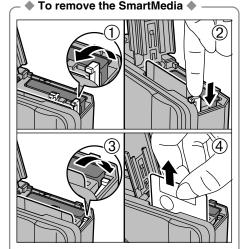
Open the battery cover, pull the SmartMedia eject button up ① and push it down ②. Then fold the SmartMedia eject button back down to its original position ③.
