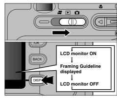
You can select the Framing Guideline function in the "**D**" still photography mode. The LCD monitor display changes each time you press the "DISP" button. Press the "DISP" button until "Framing Guideline" appears.
