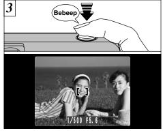
Without moving the camera, press the shutter button down halfway (AF/AE lock). Check that the AF frame on the LCD monitor has shrunk and the green viewfinder lamp has stopped flashing and is now lit.
