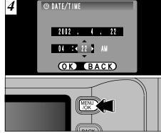
Once you have set the date and time, press the "MENU/OK" button. Pressing the "MENU/OK" button switches the camera to Photography or Plavback mode.
