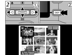
Select a frame by using "◄", "▶", "▷", "□(▲)" and " • • • • (▼)" button to move the cursor (the orange box) to the desired frame. Press the " □(▲)" or "• • • (▼)" button several times to switch to the previous page or the next page.
