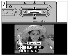
Pressing the " $[\square](\Delta)$ " or " $[\blacksquare](\nabla)$ " button during singleframe playback zooms in (enlarges) or out on a still image. When you use this function, a zoom bar is displayed. On-screen help is also displayed at the bottom of the screen.
