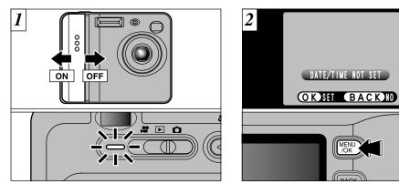
Slide the POWER switch to turn the camera on and off. When you switch the camera on, the viewfinder lamp lights (green).
