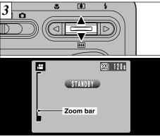
In Movie (video) mode, the lens is fixed at the wide-angle setting and only the digital zoom can be used. You can use the " $\square(\blacktriangle)$ " and " $\square(\clubsuit)$ " zoom buttons to zoom in and out. A "zoom bar" appears on the LCD monitor.
