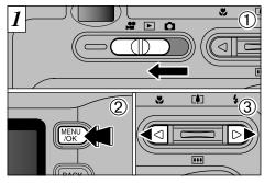
① Set the Mode switch to "#". 2 Press the "MENU/OK" button to display the menu screen.
