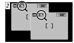
When Top 4-frame continuous shooting is set to ON, the "**Q**" icon appears on the LCD monitor. When Final 4-frame continuous shooting is set to ON, "**G**" appears on the LCD monitor. Continuous shooting continues while the shutter button is pressed down fully.
