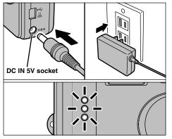
Check that the camera is switched off. Plug the AC power adapter connector into the DC IN 5V socket on the camera and then plug the adapter itself into the main power outlet.
