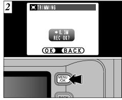
Check the size of the image being saved and then press the "MENU/OK" button. The trimmed image is added as a separate file in the last frame.
