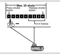
This mode allows you to release the shutter up to 25 times (at intervals as short as 0.3 seconds) and record the last 4 frames. If you take your finger off the shutter button before 25 shots have been taken, the camera records the final 4 frames shot before you released the shutter button. If there is insufficient capacity on the SmartMedia, the number of shots that could be recorded just before the shutter button was released is taken.
