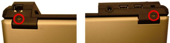
Fig. 10 Hinge cover screw.
