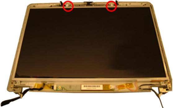
Fig. 26 The wireless LAN antenna.
